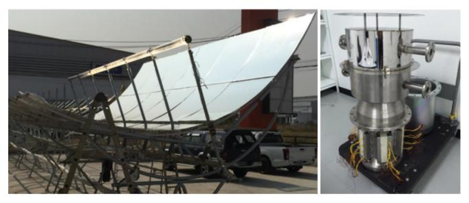
Thermal energy is harnessed and focused onto the circulating tube containing the heat transfer fluid.
